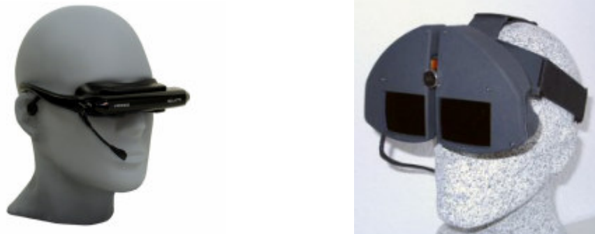
Figura 2.5: Icuiti VR920 video see-through (Izqda) y optical see through binocular r(drcha)
